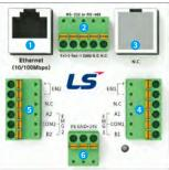
**6** Power terminal block DC 24 V input terminal block
